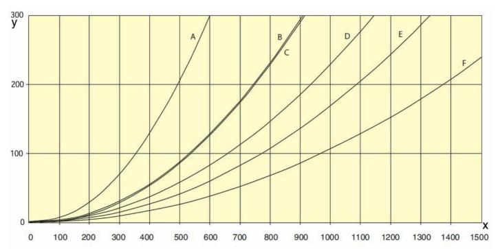
Y = Pressure drop Pa/m X = Airflow m3/h A=  $\emptyset$ 100 mm (4") on reel B=  $\emptyset$ 100 mm (4") straight C= $\emptyset$ 125 mm (5") on reel D=  $\emptyset$ 125 mm (5") straight E=  $\emptyset$ 150 mm (6") on reel F=  $\emptyset$ 150 mm (6") straight
